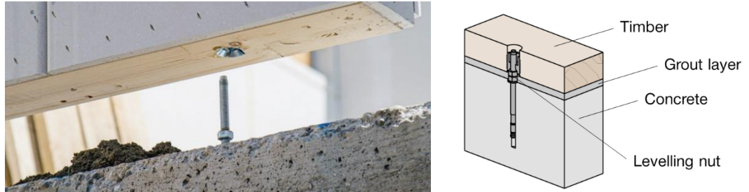
Fig. 2.6: Positioning of the HCW on top of the post-installed anchor with a levelling nut
